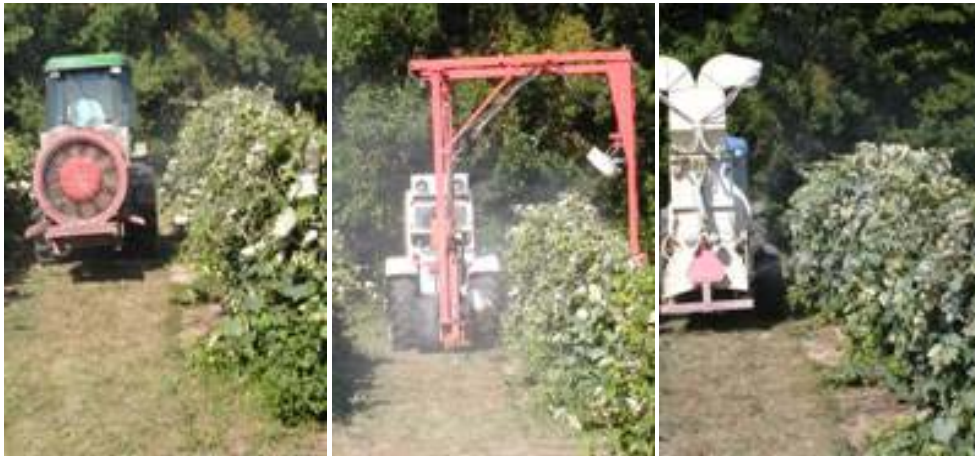
Figure 4. Sprayers used to apply spray to Concord grape canopy in August 2004. A: airblast, B: Proptec, and C: AgTec.
